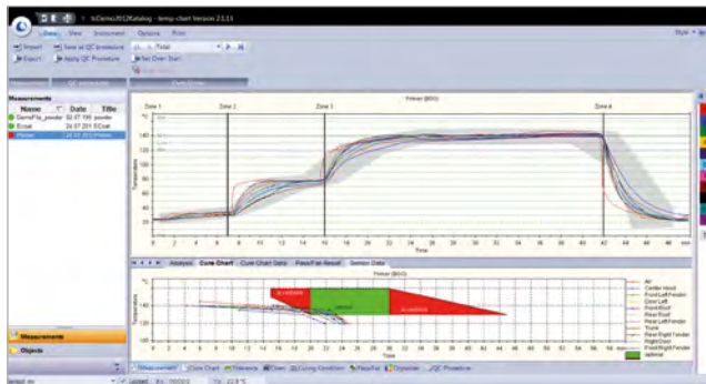
temp-gard collects temperature data in production oven.
