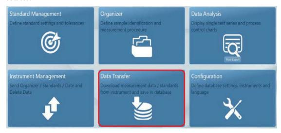
Connect the instrument to the PC and open the module **Data Transfer**.
