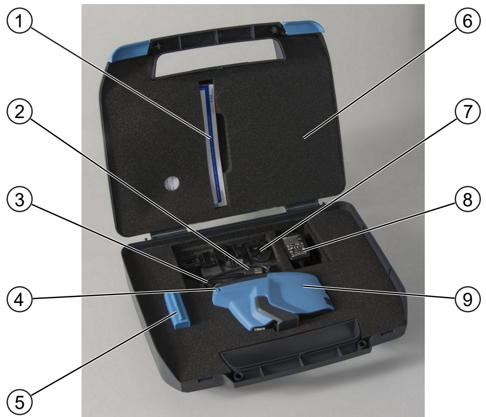
Illustration 2: Arrangement of parts in the case for instrument without docking station
