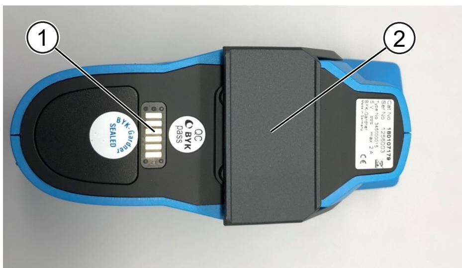
Illustration 6: Bottom view – instrument with contacts for docking station
