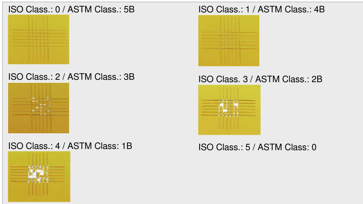
Fig. 7: Evaluation of cross-cut images
