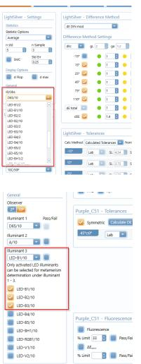
spectro2guide and color2view: Maximum 6 LED illuminants can be activated to be available for metamerism determination. In case they are added to a fluorescent standard, this standard must be remeasured to display color values for the LED illuminants. This is because both instruments store separate spectral data for each illuminant on fluorescent standards.
