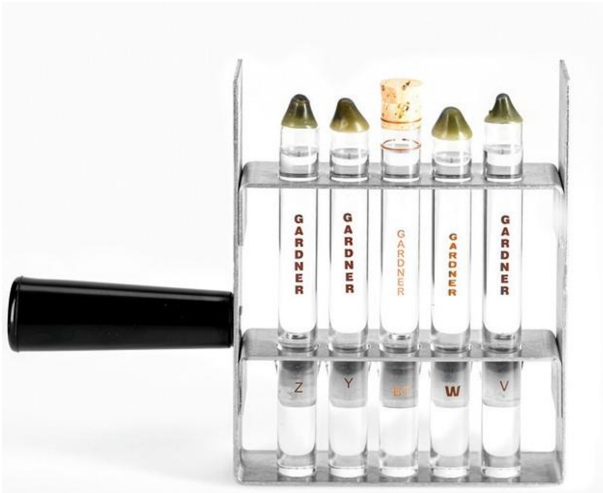
Figure 4: An array of different bubble reference tubes with a sample tube in the middle.
