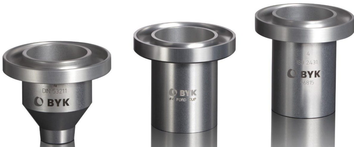
Figure 3: Overview over different types of available flow cups: DIN Cup – Ford Cup – ISO Cup.
