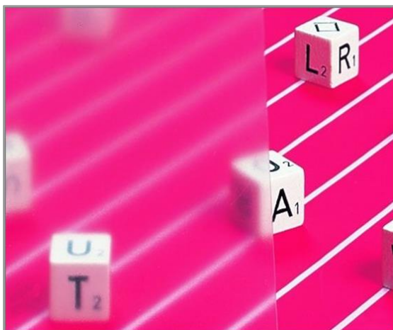
Fig. 8: Narrow angle scattering is reducing the distinctness of image (Clarity)
